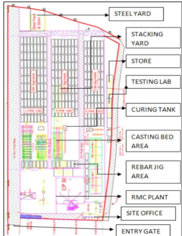
Fig. 2: Site Layout Details of Casting Yard I
