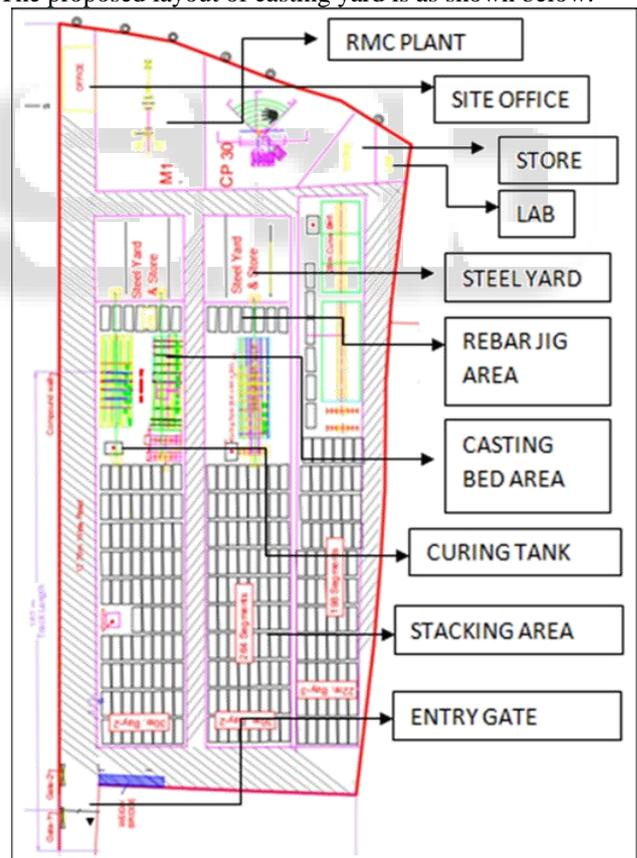
Fig. 5: Proposed Casting Yard Layout
