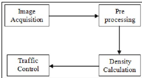
Fig. 1: Basic architecture of system for traffic density calculation
