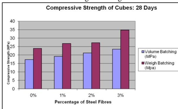
Fig. 3: Variation of compressive strength w. r. t. percentage of steel fibres
