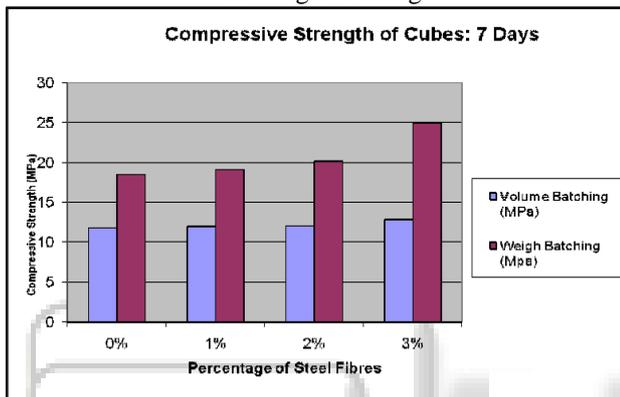
Fig. 2: Variation of compressive strength w. r. t. percentage of steel fibres
