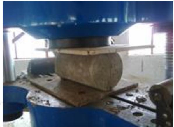
Photo 4: Specimen testing for split tensile strength
