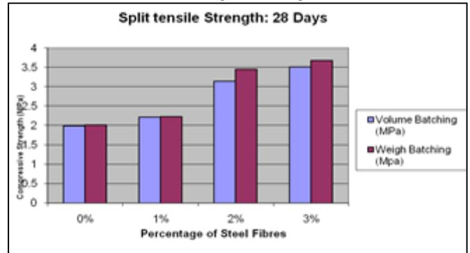
Fig. 4: Variation of compressive strength w. r. t. percentage of steel fibres
