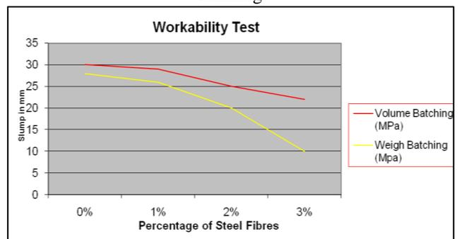
Fig. 1: Variation of slump w. r. t. percentage of steel fibres
