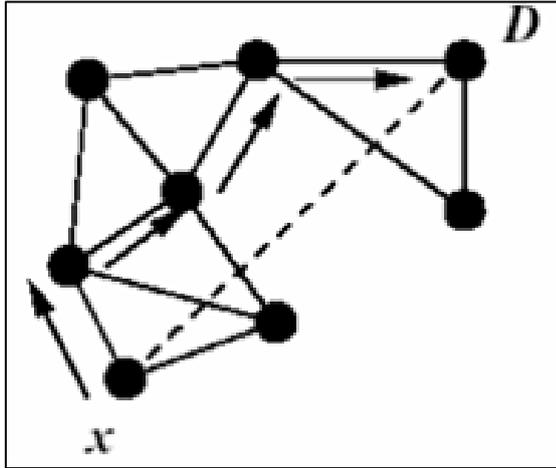
Fig 3. Perimeter Forwarding:  $x$  is the node where Greedy forwarding failed. Algorithm uses right hand rule to forward packets.
