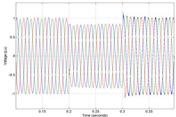
Fig. 5: Three phase voltage sag mitigation waveform with UPQC without neural network
