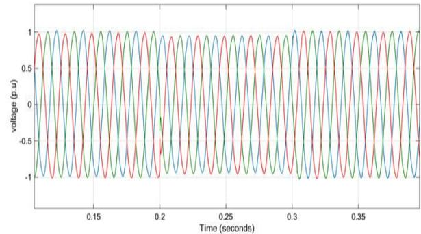
Fig. 4: Three phase voltage sag mitigation waveform by neural network based UPQC
