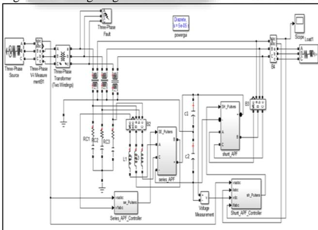
Fig. 3: Simulink model of three phase system with three phase fault
