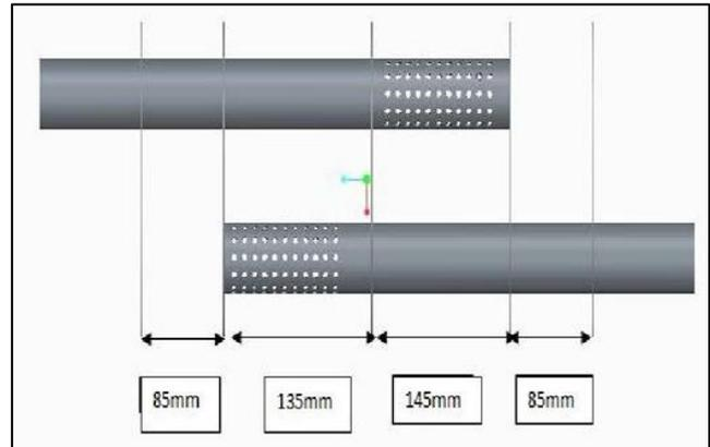
Fig. 1: Top view of Muffler I
