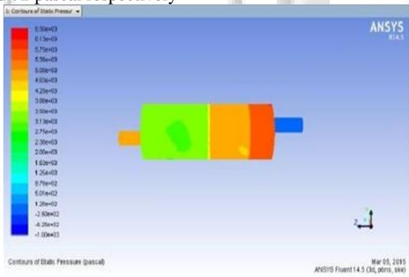
Fig. 5: Pressure distribution in Muffler I
