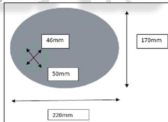
Fig. 2: front view of muffler
