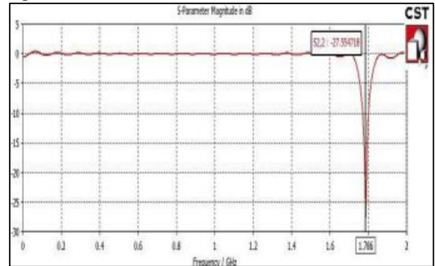
Fig. 6: Simulated Return Loss vs. Frequency of Simple RMPA is 27.554dB at 1.786GHz
