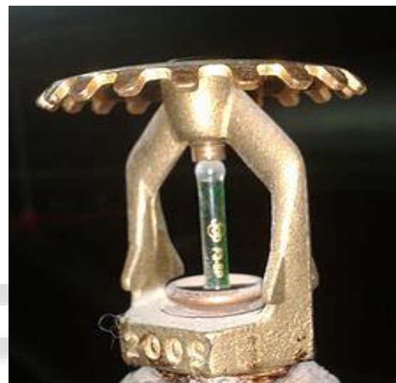
Fig. 6: A sprinkler with a green bulb indicating a liquid alcohol
