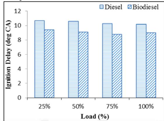
Fig. 3: Variation of ignition delay with load (%)
