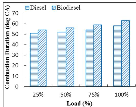
Fig. 4: Variation of combustion duration with load (%)
