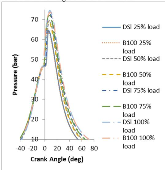
Fig. 2: Variation of in-cylinder peak pressure with CA
