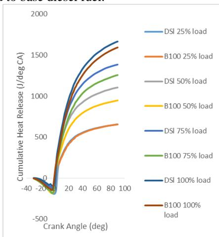
Fig. 6: Variation of cumulative heat release with CA
