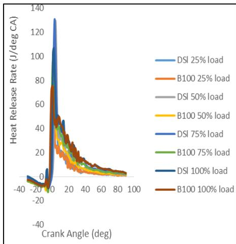
Fig. 5: Variation of heat release rate with CA
