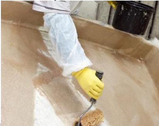
Fig. 3: Hand lay-up method
