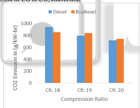
Fig. 6: Variation of CO<sub>2</sub> emission with different CR
