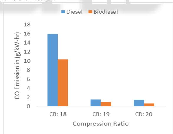
Fig. 4: Variation of CO emission with different CR
