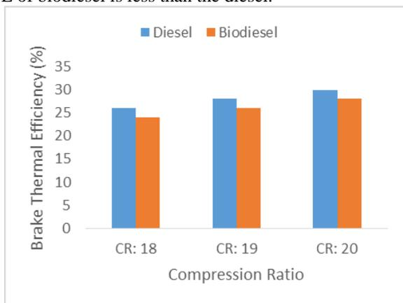
Fig. 2: Variation of brake thermal efficiency with different CR
