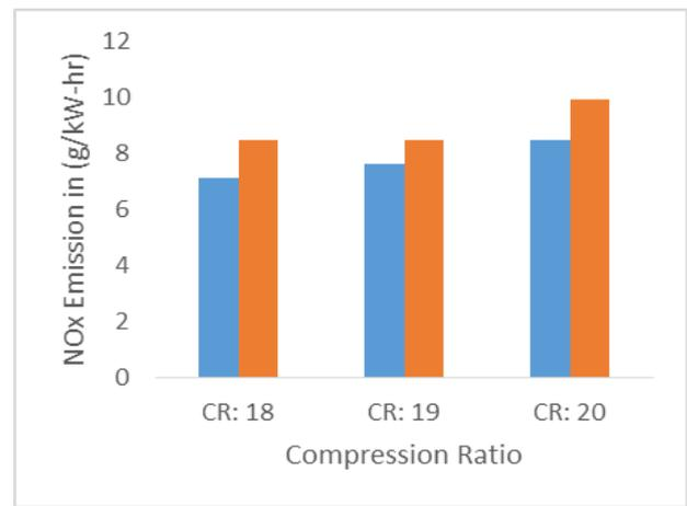
Fig. 7: Variation of NO<sub>x</sub> emission with different CR
