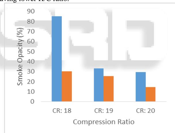
Fig. 8: Variation of smoke opacity with different CR
