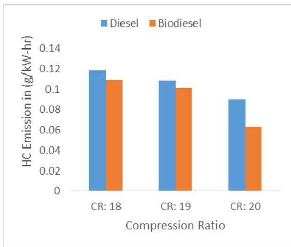
Fig. 5: Variation of HC emission with different CR
