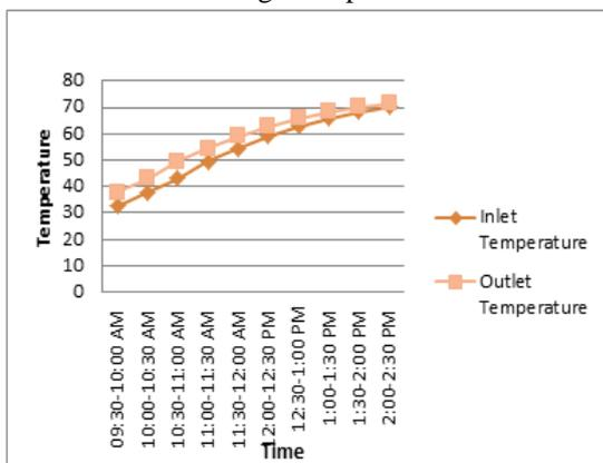
Fig. 4: Variation in Temperature with Time at Flow Rate of 2.66 Ltr/Min
