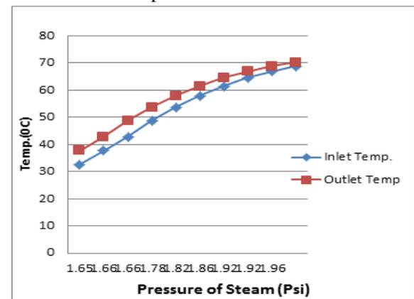
Fig. 7: Variation in Steam Pressure with Inlet and Outlet Temperature at 2.66 LPM
