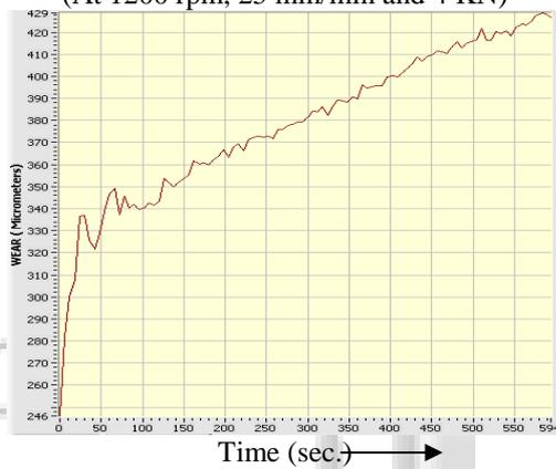
Fig.20: Wear Rate curve for specimen no.7
