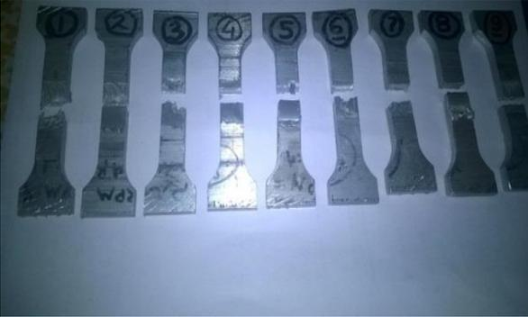
Fig. 5: Sample after Tensile Testing FSW AA 6063 samples
