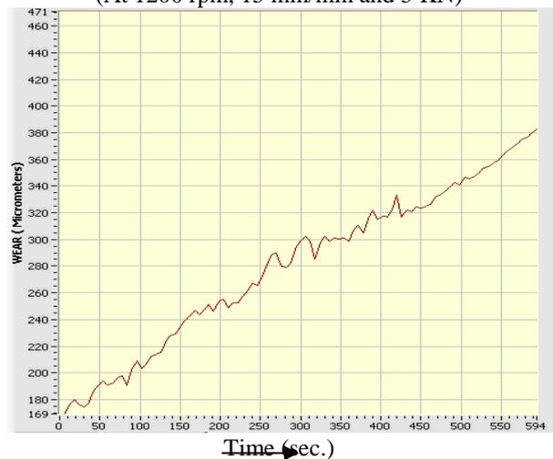
Fig. 18: Wear Rate curve for specimen no.5 (At 1200 rpm, 20 mm/min and 6 KN)
