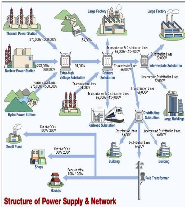
Fig. 4: Structure of Power Supply & Network
