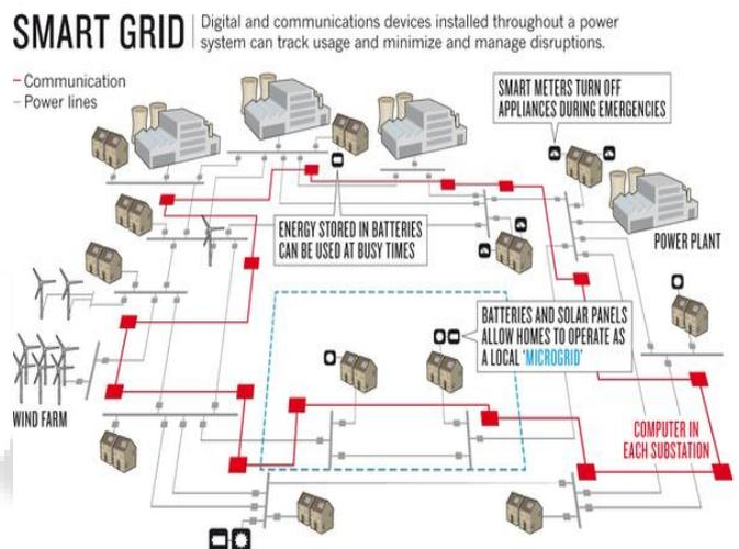
Fig. 1: Block Diagram of Smart Grid
