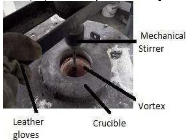
Fig. 1: Set Up of Stir Casting
