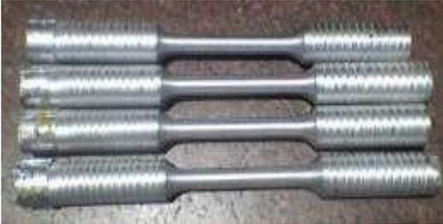
Fig. 3: Specimens Prepared For Tensile Testing,
