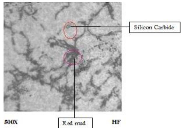
Fig. 6(b): Micro Structural Studies of Aluminium Alloy 7075+4% SiC+4% Red Mud
