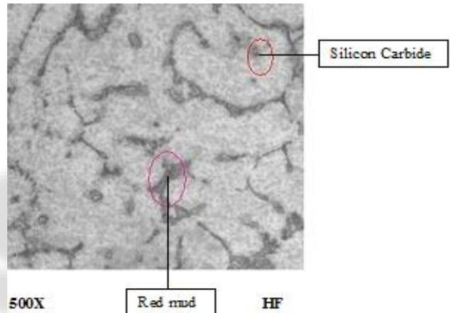
Fig. 6(a): Micro Structural Studies of Aluminium Alloy 7075+6% SiC+2% Red Mud
