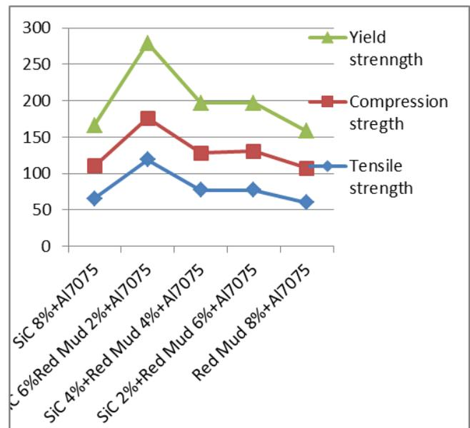
Fig. 7: variations in tensile, compressive and yield strength for different wt% composition of SiC and red mud composite.
