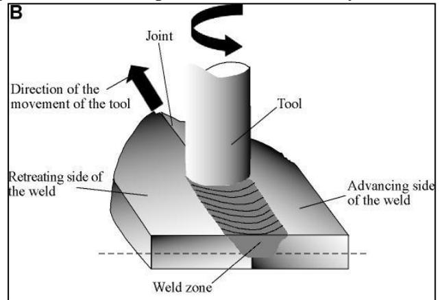
Fig. 1: Process of Friction Stir Welding
