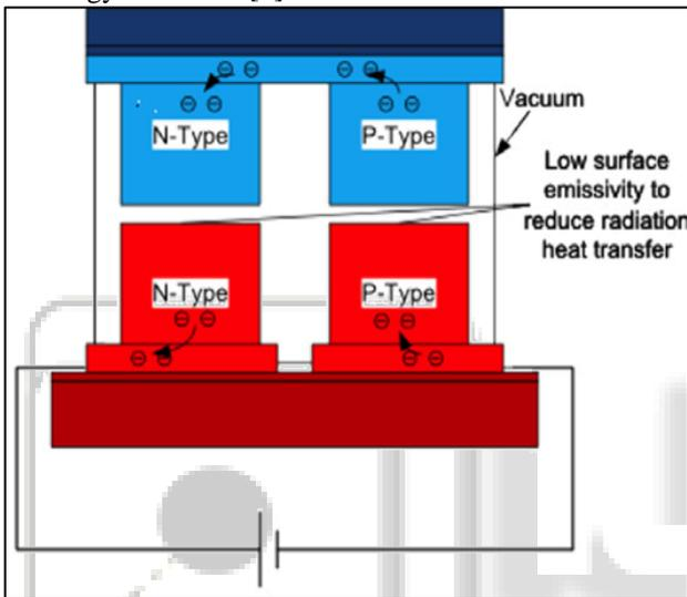
Fig. 6: Thermo tunneling refrigeration
