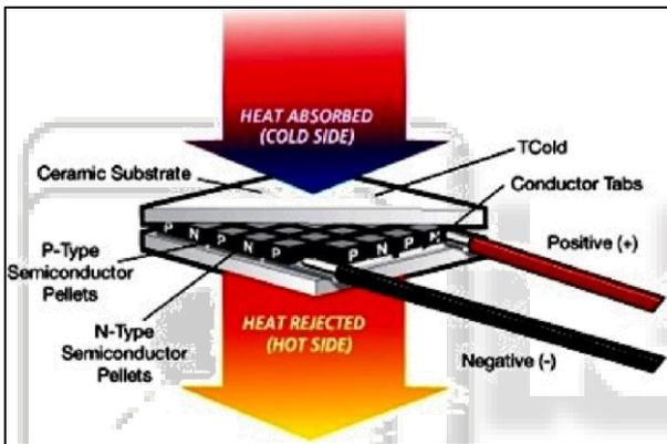
Fig. 4: Thermoelectric module assembly
