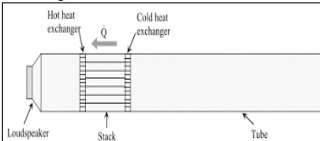
Fig. 2: Simple thermo acoustic refrigerator
