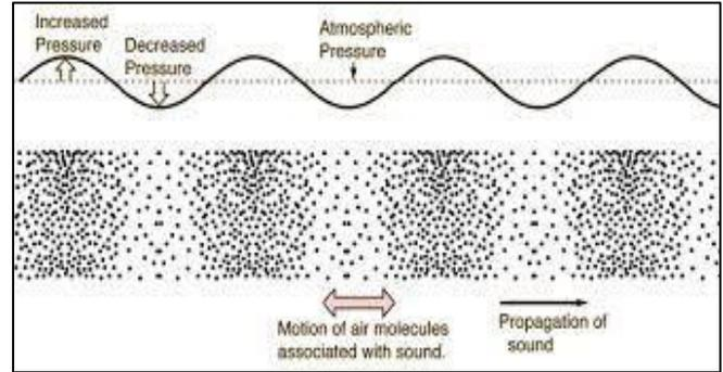
Fig. 3: Pressure variation and displacement of sound waves.
