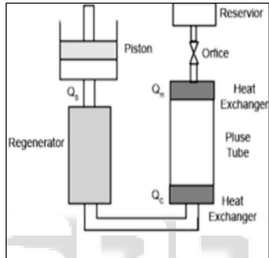
Fig. 7: Basic pulse tube refrigerator
