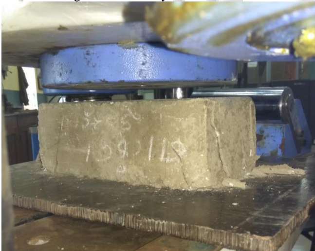
Fig. 5: Fly Ash bricks after Test
