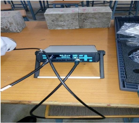
Fig. 3: ultrasonic plus velocity test.
