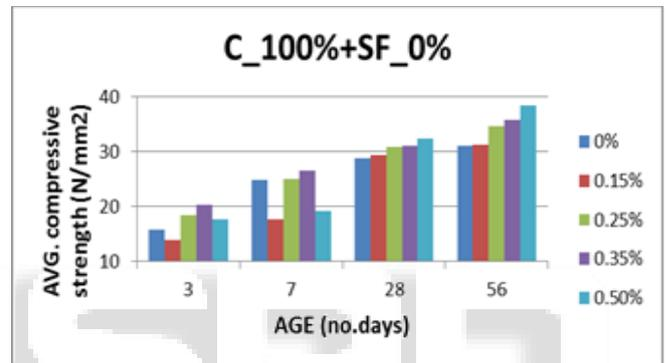
Fig. 4: Compressive Strength for C100% SF0%
