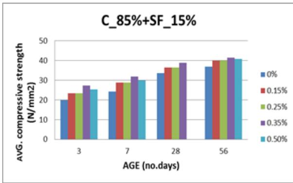
Fig. 6: Compressive Strength for C85% SF15%
