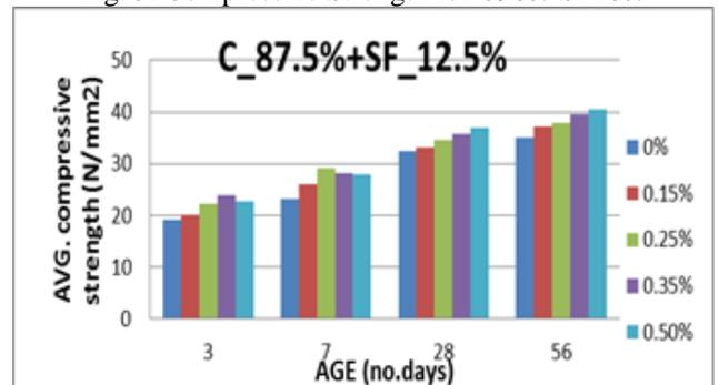
Fig. 6: Compressive Strength for C87.5% SF12.5%
