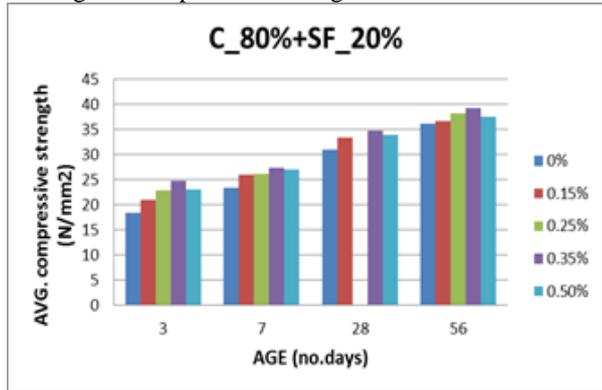
Fig. 7: Compressive Strength for C80% SF20%
