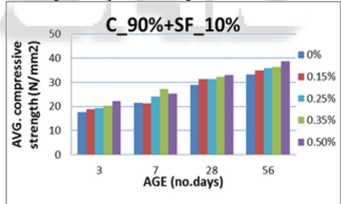
Fig. 5: Compressive Strength for C90% SF10%
