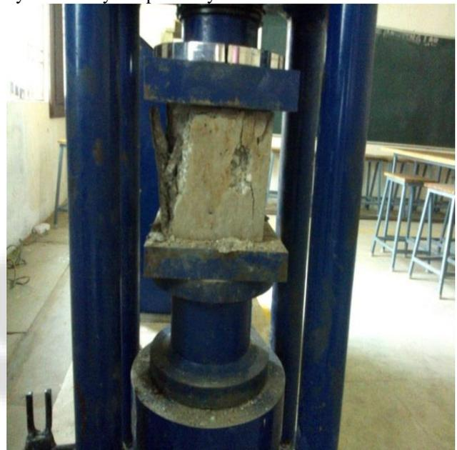
Fig. 2: Testing of cubes for compressive strength
