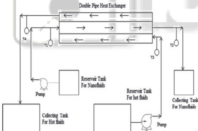
Fig. 1: Experimental setup of concentric tube heat exchanger [4]
