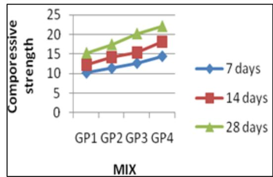
Fig. 5: Compressive Strength vs. Mix at 60°C
