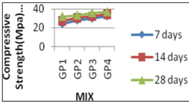
Fig. 3: Compressive Strength vs. Mix at 60°C
