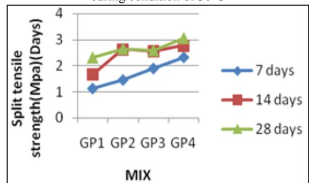
Fig. 6: Split Tensile Strength vs. Mix at 30°C
