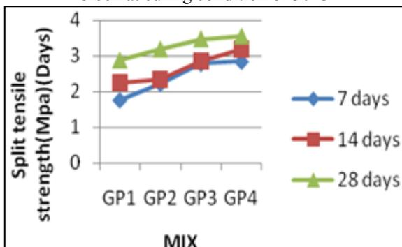
Fig. 9: Split Tensile Strength vs. Mix at 60°C
