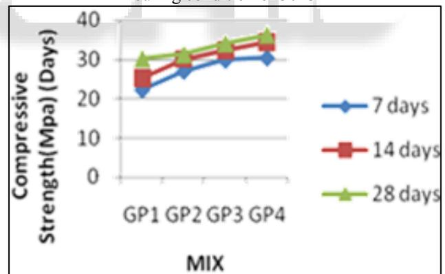
Fig. 2: Compressive Strength vs. Mix at 30°C
