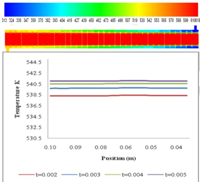
Fig. 4: Temperature variation across Outlet for varying Fin thickness.
