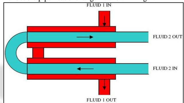
Fig. 1: Double pipe heat exchanger
