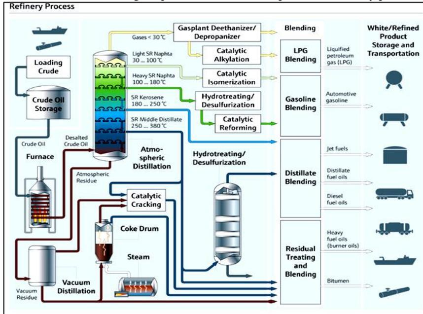
Fig. 2: Refinery process
