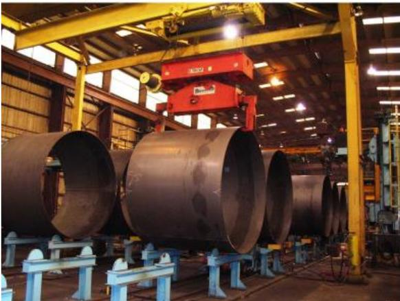
Fig. 1: Overhead Crane Used in Material Handling
