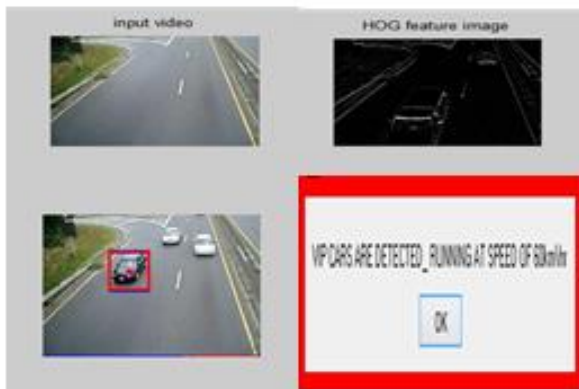
Fig. 10: Simulated result video vip car and speed detected using matlab
