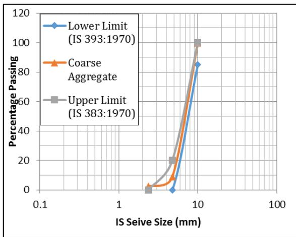
Fig. 2: Grading curve of 10 mm Coarse aggregate
