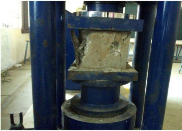
Fig. 4: Testing of cubes for Compressive strength
