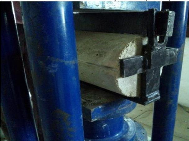
Fig. 5: Testing of cylinders for Split tensile strength
