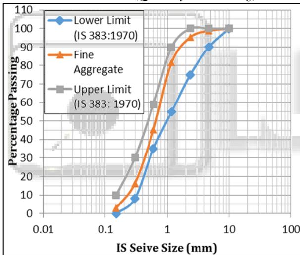
Fig. 3: Grading curve of Fine aggregate
