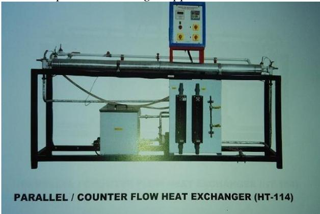
The apparatus consists of a concentric tube heat exchanger. The hot water flows through inner tube and cold water flows through outer tubes. Direction of cold fluid flow can be changed from parallel to counter to hot water so that unit can be operated as parallel or counter flow heat exchanger. For flow measurement Rota meters are provided. A magnetic drive pump is used to circulate the hot water from a recycled type water tank, which is fitted with heaters and digital temperature controller.
