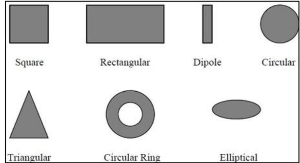
Fig. 2: Common shapes of microstrip patch elements
