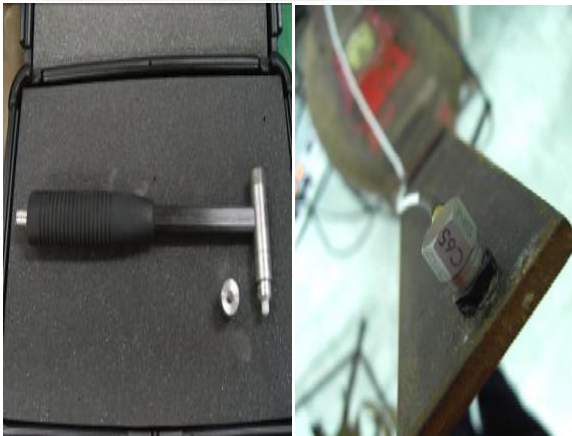
Fig. 1: Transducer used for excitation (left) and response measurement (right).
