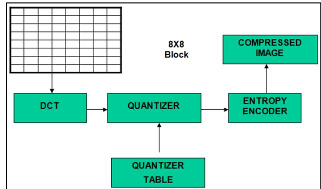
Fig. 1: DCT compression technique [1] [2]
