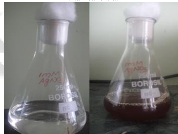
Fig. 2a: AgNO 3 solution without adding the plant extract of Neem (Control), After the addition of AgNO 3 into the neem leaf extracts (Test)
