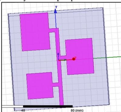
Fig. 6: Geometry of Rectangular Shaped Log periodic antenna
