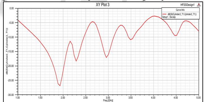
Fig. 9: Return loss versus frequency plot
