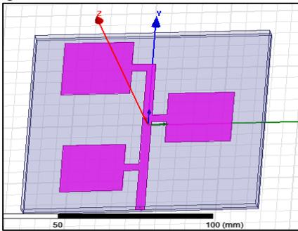
Fig. 4: Geometry of Square Shaped Log periodic antenna
