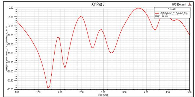
Fig. 7: Return Loss versus Frequency Plot
