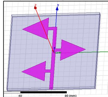
Fig. 8: Geometry of Triangular Shaped Log periodic antenna
