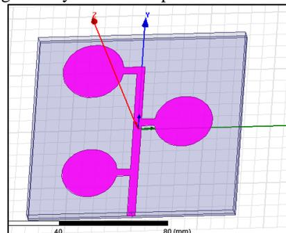
Fig. 10: Geometry of Circular Shaped Log periodic antenna
