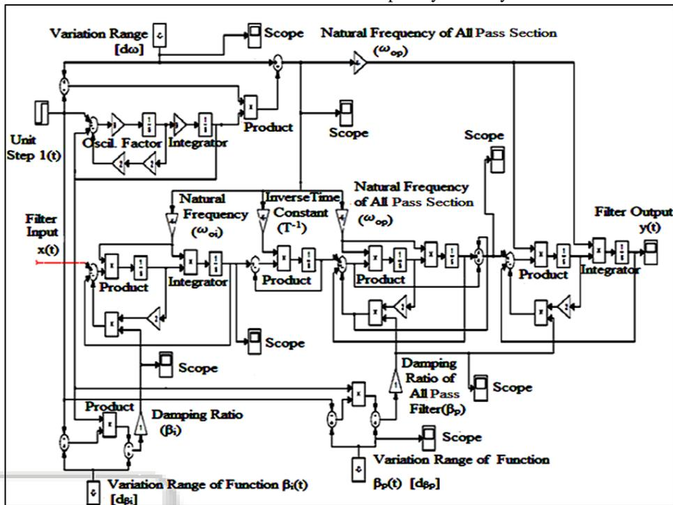
Fig. 4: Model of third order phase compensated time varying chebyshev filter
