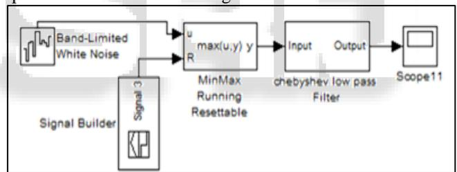
Fig. 5: Block diagram to generate noisy signal
