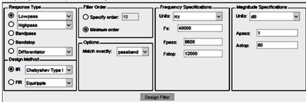
Fig. 6: Specification taken for designing low pass chebyshev filter using FDA Tool
