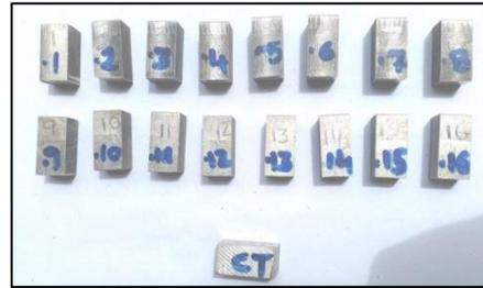
Fig. 2(d): Test-pieces who surface Roughness is measured
