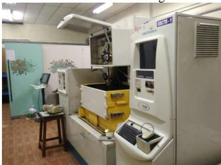
Fig. 2(a): Electronica Ultracut S2 Wire-EDM
