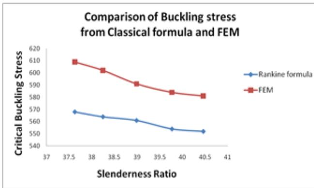
Fig. 11: Experimental and Simulation Result the Reduced cross section of Connecting rod
