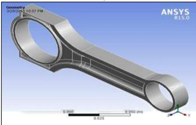
Fig. 5: CAD Model of Connecting Rod width 26mm
