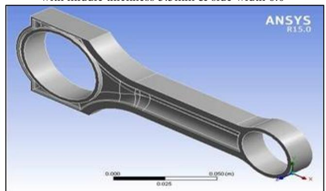
Fig. 9: CAD Model of Connecting Rod total width 25mm with middle thickness 5.4mm & side width 6.1
