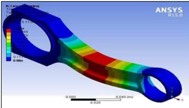
Fig. 17: Critical Buckling of I-section Connecting rod width 23mm
