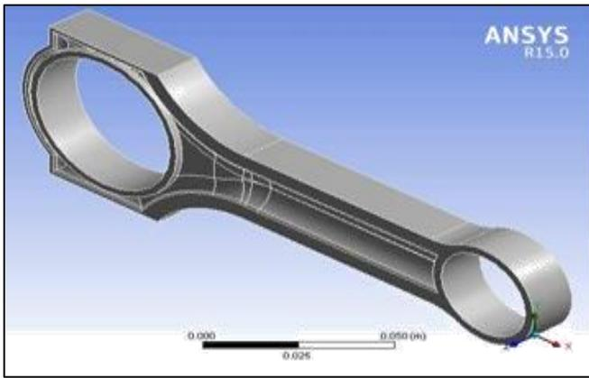
Fig. 10: CAD Model of Connecting Rod total width 24mm with middle thickness 5.3mm & side width 6.2
