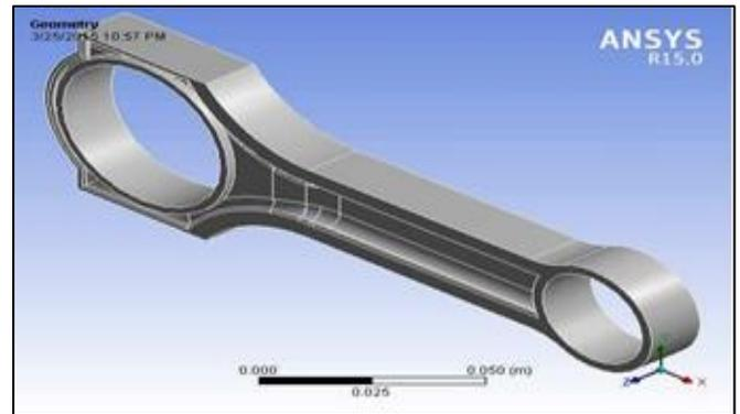
Fig. 7: CAD Model of Connecting Rod width 24mm
