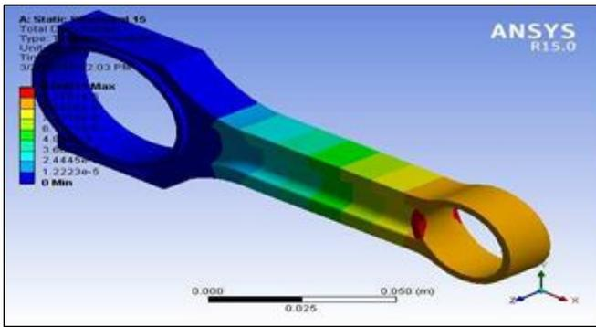
Fig. 16: Total Deformation of I-section Connecting rod width 25mm
