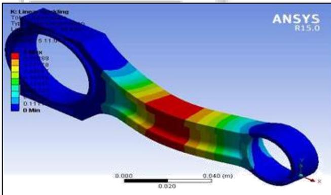
Fig. 18: Critical Buckling of I-section Connecting rod width 23mm
