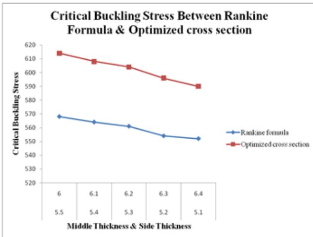
Fig. 21: Rankine formula and Simulation Result of the optimized cross section of Connecting rod.
