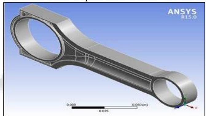
Fig. 8: CAD Model of Connecting Rod total width 26mm with middle thickness 5.5mm & side width 6.0
