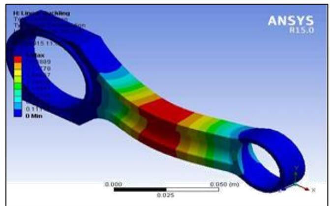
Fig. 24: Critical Buckling of Optimized I- Section Connecting rod width 25mm and different middle thickness & side width
