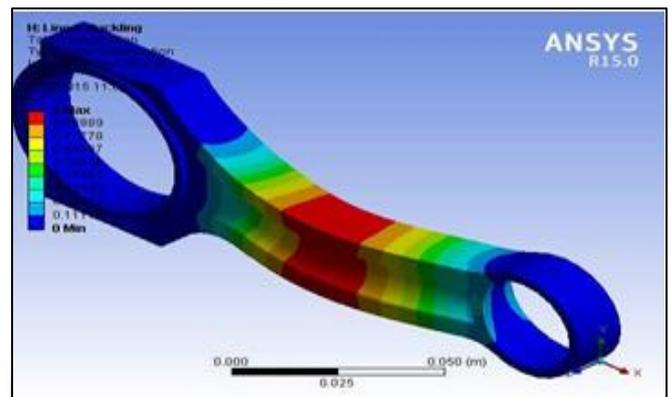
Fig. 25: Critical Buckling of Optimized I- Section Connecting rod width 24mm and different middle thickness & side width
