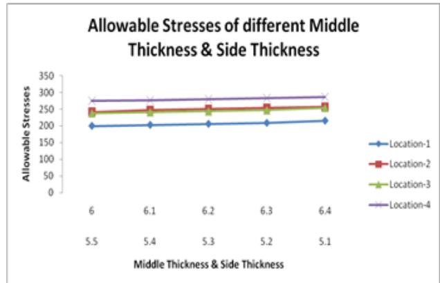
Fig. 19: Optimization result of Allowable stress of optimized-Cross Section of the Connecting rod of Middle Thickness & Side Thickness.
