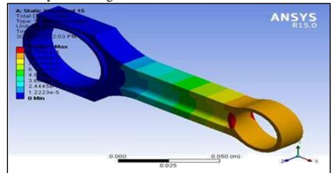
Fig. 15: Total Deformation of I-section Connecting rod width 26mm
