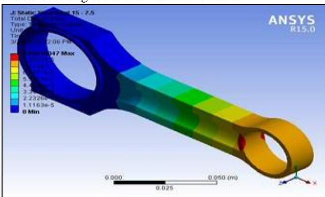
Fig. 22: Total Deformation of Optimized I- Section Connecting rod width 26mm and different middle thickness & side width
