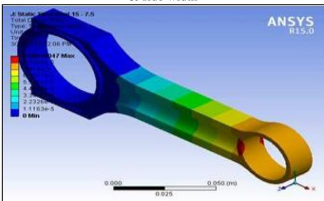
Fig. 23: Total Deformation of Optimized I- Section Connecting rod width 25mm and different middle thickness & side width
