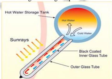
Fig. 9: Glass –Glass Evacuated Tube Collector
