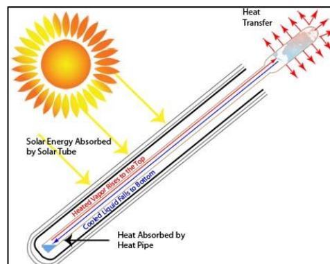
Fig. 2: Construction of Evacuated Heat Pipe
