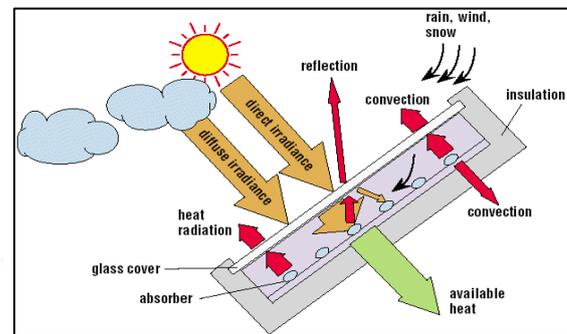
Fig. 7: Flat Plate Collector
