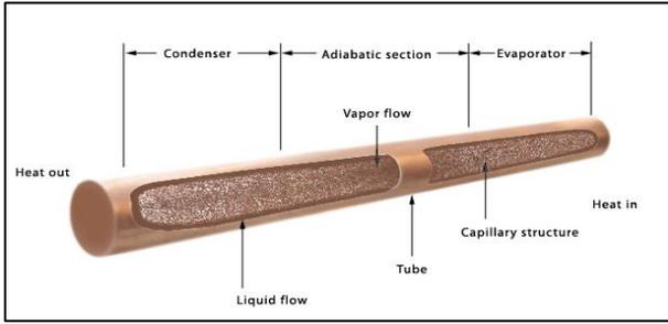
Fig. 5: Section of Heat Pipes
