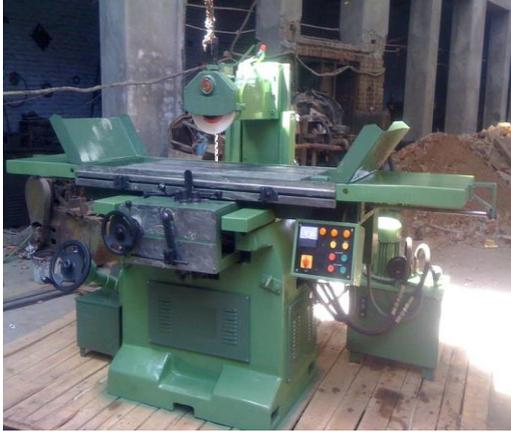
Fig. 1: Photographic view of surface grinding machine
