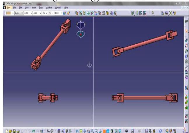
Fig. 3: Multiple views of steering yoke in CATIA V5 interface
