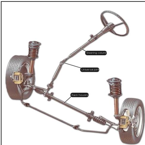
Fig. 1: A typical rack-and-pinion steering layout, showing how the rack acts directly on the road-wheel steering arms.
