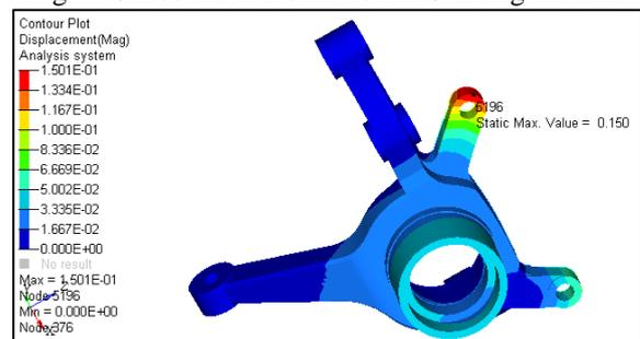
Fig. 5: Stress and Deformation in Steering knuckle
