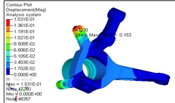
Fig. 8: Stress and Deformation in 3<sup>rd</sup> (Final) Iteration
