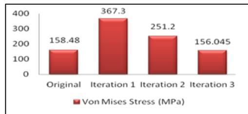
Fig. 12: Stress Change in Steering Knuckle
