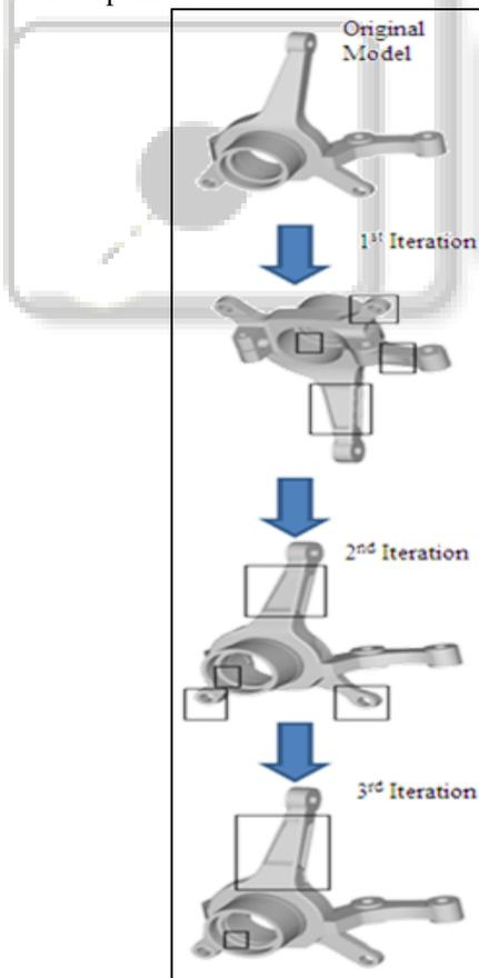
Fig. 6: Structural Optimization of Steering Knuckle
