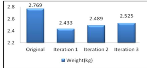
Fig. 13: Weight Change in Steering Knuckle
