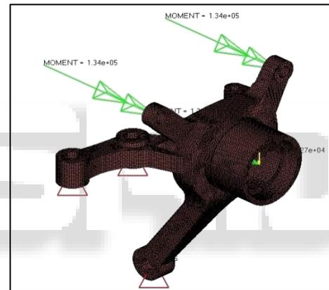
Fig. 3: Details of Loading and Boundary Condition
