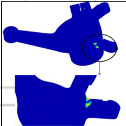
Fig. 11: Fatigue Location of Steering Knuckle
