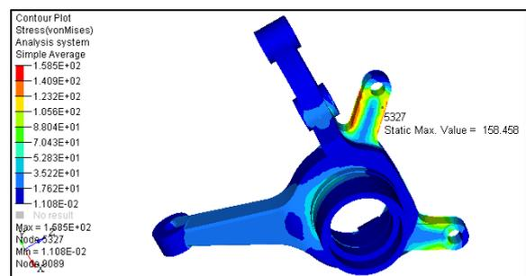
Fig. 4: Stress and Deformation in Steering knuckle
