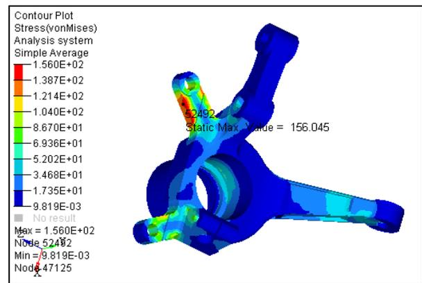
Fig. 7: Stress and Deformation in 3<sup>rd</sup> (Final) Iteration
