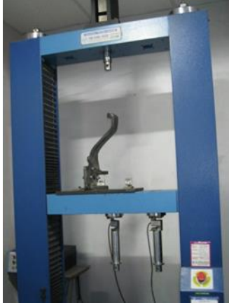
Fig. 16: Test setup for physical experimentation to calculate stiffness
