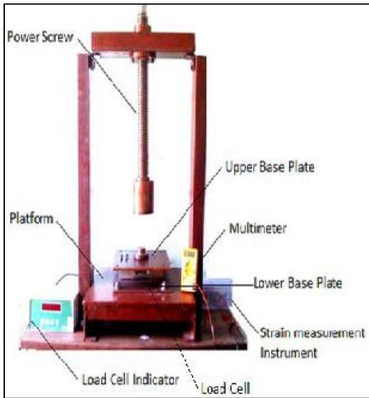
Fig. 3: Experimental set up
