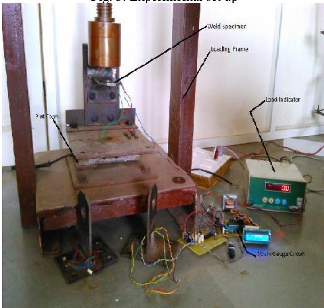
Fig. 4: Welded Joint Specimen Mounted on Experimental Setup
