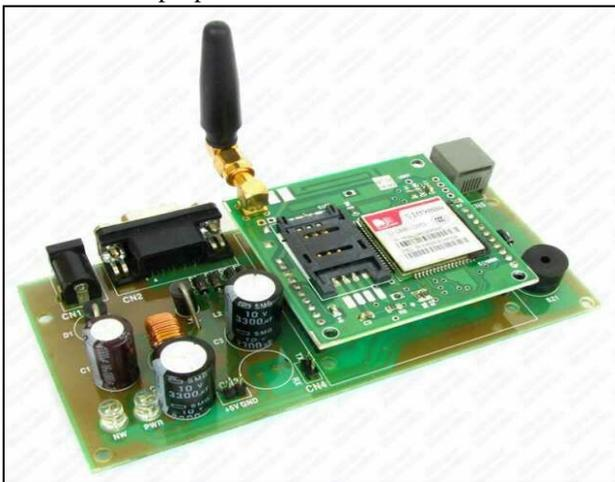
Fig. 3: GSM Modem
