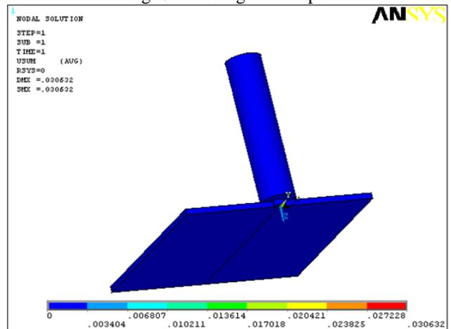
Fig. 9: Nodal solution of displacement
