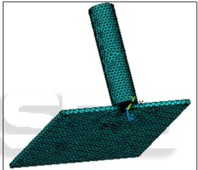
Fig. 8: Meshing the sample
