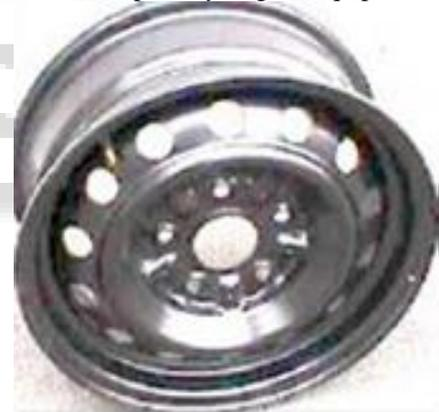
Fig. 6: Steel Disc Wheel
