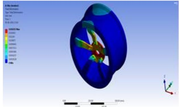
Fig. 8: Total deformation
