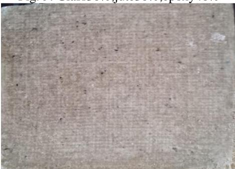
Fig. 10: Glass20%, jute30%, epoxy40%, ash10%
