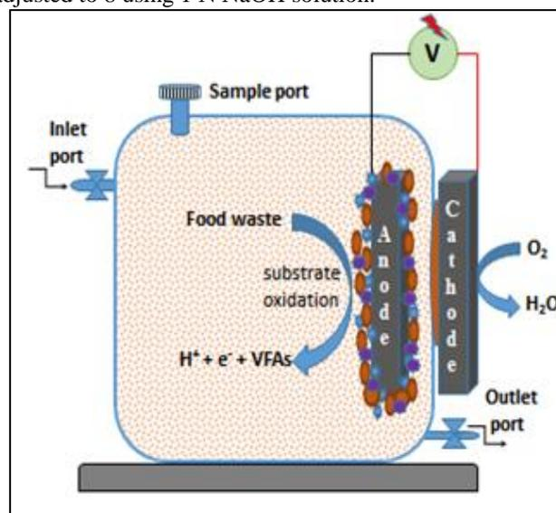
Fig. 1: Schematic illustration of MFC architecture
