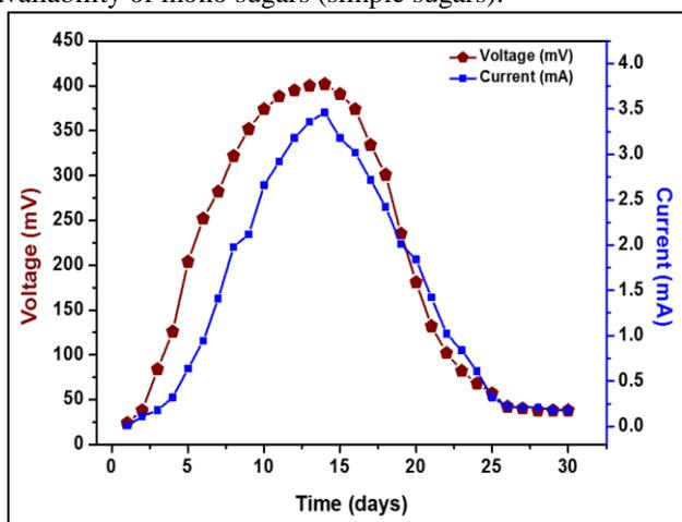
Fig. 2: Voltage and current generation with respective of time during MFC operation
