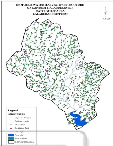
Fig. 6: Water Harvesting structures (check dams, boulder checks, check dams) map
