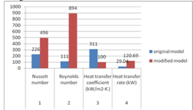
Fig. 9: Comparison of CFD analysis output parameters of original and modified models of rectangular fins.
