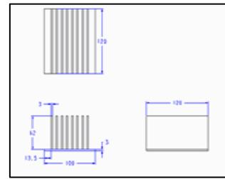
Fig. 1(a): CAD model Original Fin
