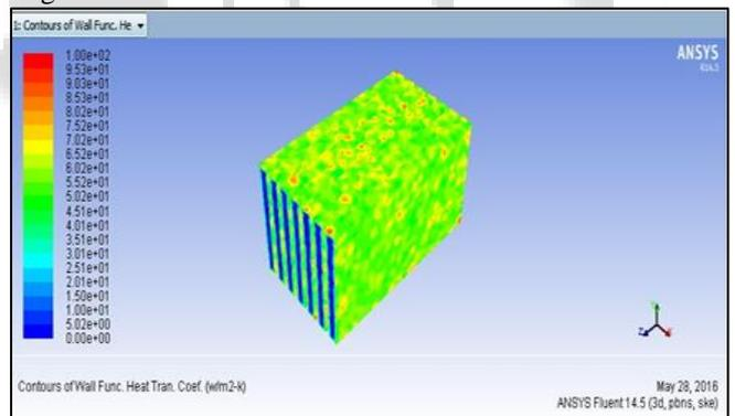
Fig. 7(a): Heat Transfer Coefficient For Original Model
