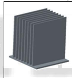
Fig. 2(b): PRO-E model Modified Fin
