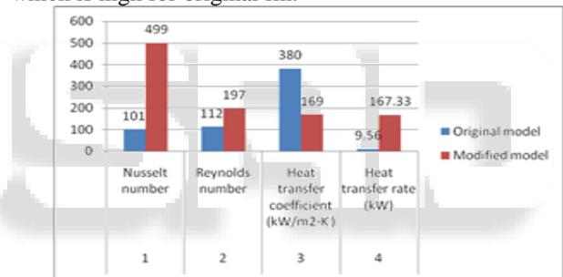
Fig. 4: Comparison of CFD analysis output parameters of original and modified models of solid fin.
