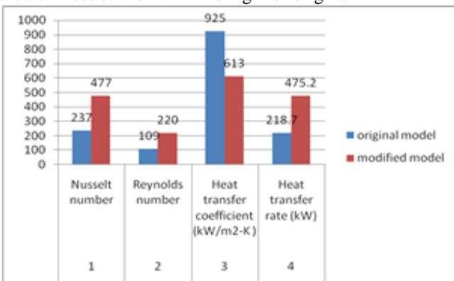
Fig. 6: Comparison of CFD analysis output parameters of original and modified models of elliptical fin.
