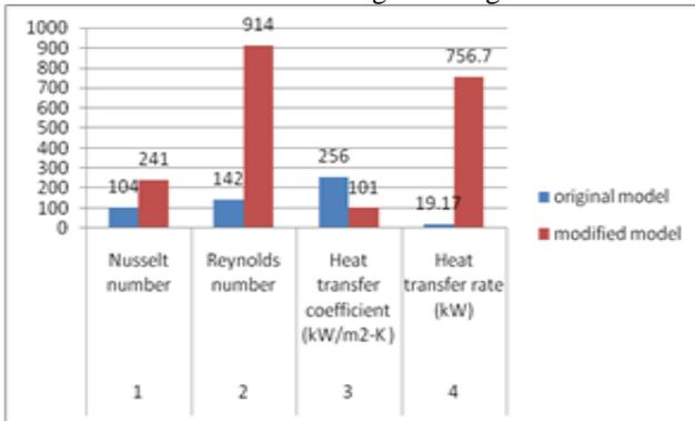
Fig. 8: Comparison of CFD analysis output parameters of original and modified models of circular fin.
