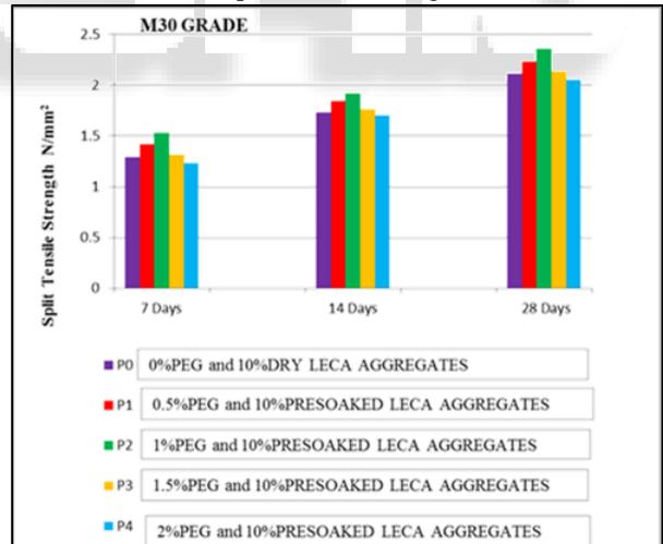
Fig. 4: Split Tensile Strength for Different designation
