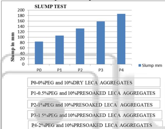
Fig. 1: Slump Value for Different Designations
