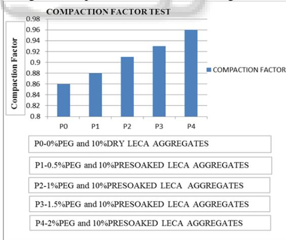
Fig. 2: Compaction Factor Value for Different Designations
