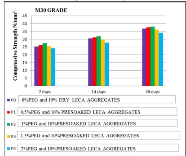
Fig. 3: Compressive Strength for Different designation
