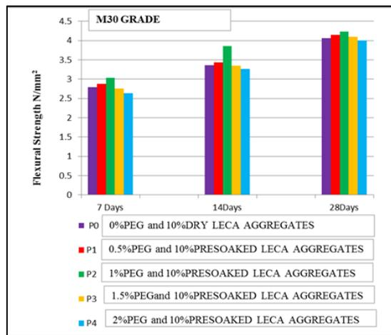
Fig. 5: Flexural Strength for Different Designations.
