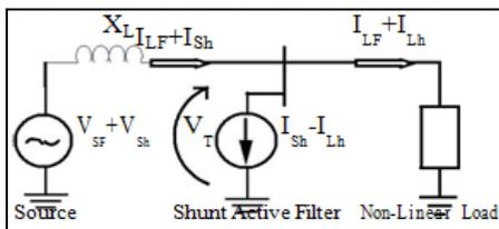
Fig. 3: Principle of Shunt Current Compensation
