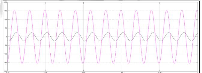
Fig. 11: Voltage and Current are in Phase Using PI Controller
