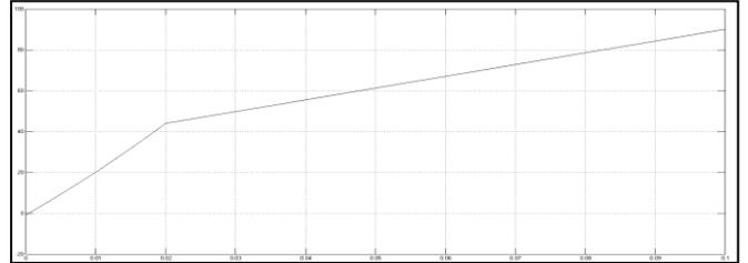
Fig. 10: DC Capacitor Voltage During Switch-on Response with PI Controller
