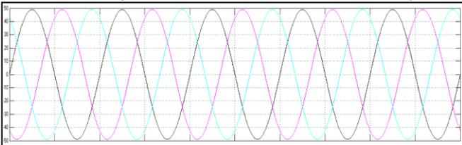
Fig. 7: source voltage waveform of the system
