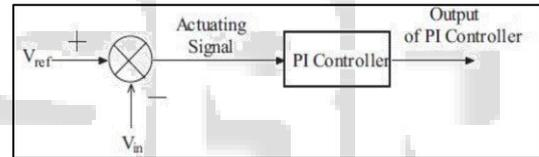
Fig. 4: APF Control Scheme with PI controller
