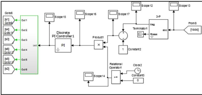
Fig. 6: Subsystem used for Producing 6 Pulses of Inverter
