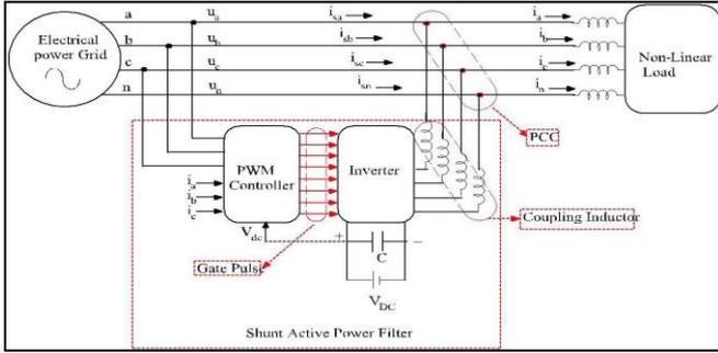
Fig. 1: Shunt Active Power Filters Topology
