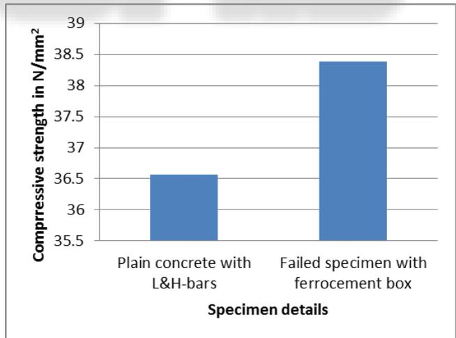
Fig. 3:(c) showing variation in compressive strength between series 4 and failed specimen provided with Ferro-cement box
