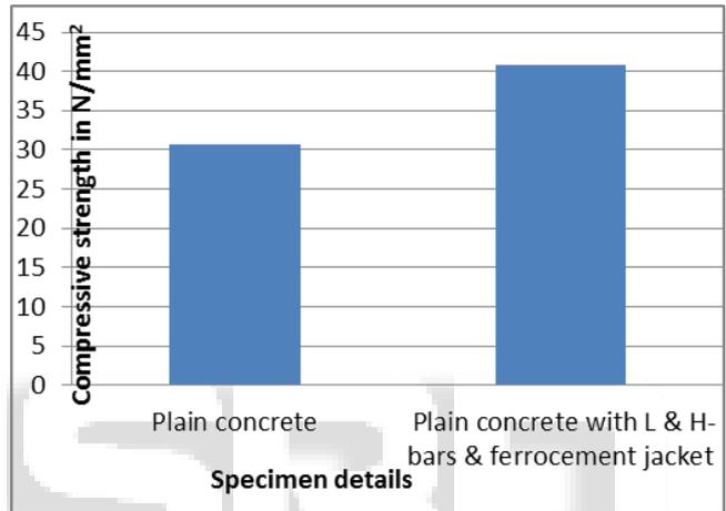
Fig. 2: showing variation in compressive strength between series 1 & 3
