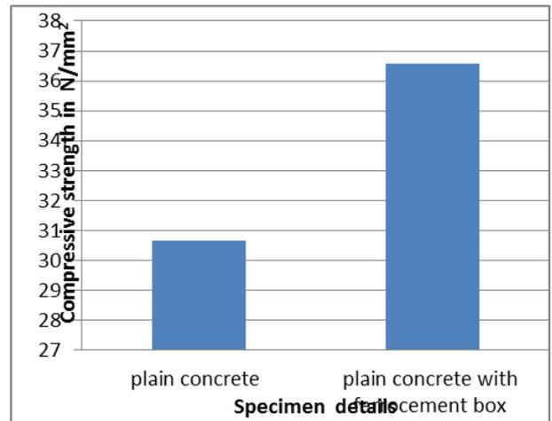
Fig. 1: showing variation in compressive strength between series 1 & 2
